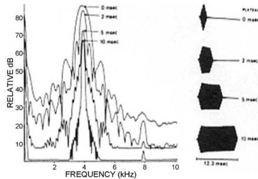
**Figure 3** The effects of tone-burst duration on spectrum. Reprinted from Burkard (1984)<sup>9</sup> with the permission of Elsevier.
