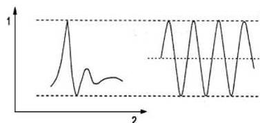
**Figure 4** A schematic of peak-to-peak peak-equivalent sound pressure level measurement. (1 indicates the amplitude axis; 2 indicates the time axis.) The authors thank the International Electrotechnical Commission for permission to reproduce information from its International Standard IEC 60645-3 ed. 2.0 (2007).
